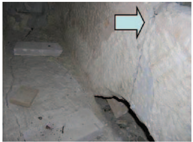
FIG. 3. The interior surface of the sarcophagus is covered by a thin layer of lime. The sampling area was the top edge of a vertical fracture.
