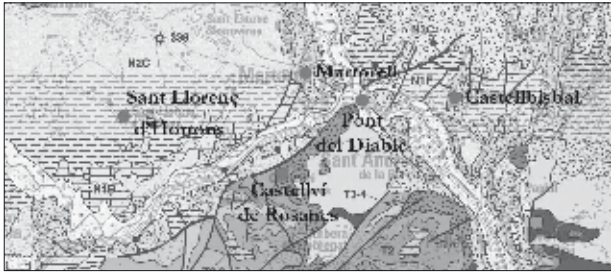
FIG. 4. Geological map of the area showing the location of the bridge and the nearby localities (ICC 2002, scale: 1.250.000). Key: N1: Lower Miocene; N2: Middle/Upper Miocene; N3: Upper Miocene; T1: Lower Triassic; T2/T3: Middle/Upper Triassic.
