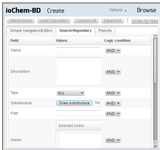
Figure 5. CREATE search panel allows users to define multiple search criteria using boolean logic. Such queries range from administrative metadata, chemical related terms and chemical substructure.
