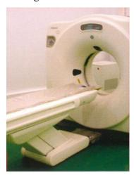
A CT equipment calibrated for drycured ham is available in the facilities of IRTA-Center (Monells, Girona). This technology enables to visualize into a single piece both saltdistribution and dehydration along the process. It also allows monitoring geometrical changes of the pieces. CT is a very useful tool to define at pilot scale the most suitable process
