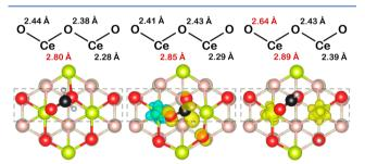
**Figure 4.** (Top) Most relevant Ce-O distances in Å for the initial, transition, and final states of formaldehyde decomposition on CeO<sub>2</sub> at PBE+U (U = 3.5 eV) level. (Bottom) Electron localization in the initial, transition, and final states. Same color code as in Figure 1.
