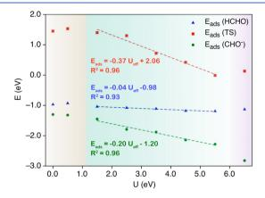
**Figure 5.** Adsorption energy of formaldehyde (blue), transition step for first hydrogen stripping (red), and final state (green), all with respect to gas-phase formaldehyde and the bare  $Fe_2O_3$  surface, as a function of U. The background color indicates when the electron is properly localized in the Fe center (turquoise) and when spin-crossing is observed (purple). Notably, the dependences of the kinetic and thermodynamic terms are different.
