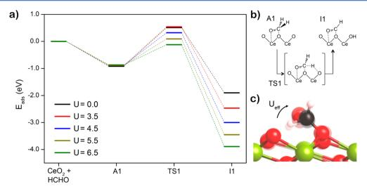
Figure 1. (a) Adsorption of formaldehyde (A1) on the CeO<sub>2</sub>(111) regular surface and first hydrogen stripping to CHO and OH (I1). (b) Reaction scheme for this elementary step. (c) Overlaid structures of TS1 for the different *U* values. Red stands for oxygen, yellow for cerium, black carbon, and white hydrogen.
