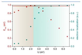
**Figure 3.** Reduction energy  $(E_{red}, red)$  and electron localization (turquoise) as a function of the Hubbard U parameter. The horizontal solid line accounts for the screened hybrid HSE06  $E_{red}$  result. The background color indicates when the electron is properly localized in the Ce center (turquoise).
