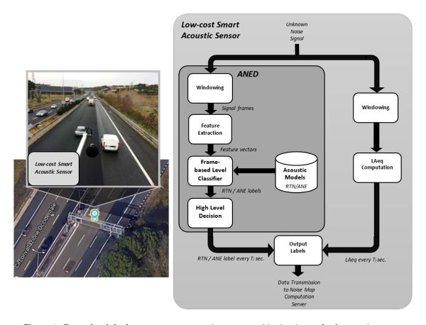
**Figure 1.** Example of the low-cost smart acoustic sensor positioning in a suburban environment (pictures loaned courtesy of ANAS S.p.A.) and the ANED functional block diagram.
