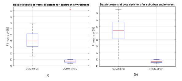
**Figure 4.** Boxplots of the classifiers' performance at the (a) frame level and (b) high level on the suburban environment considering the binary-based GMM and UGMM classifiers and MFCC features, as well as following a leave-one-out cross-validation scheme.
