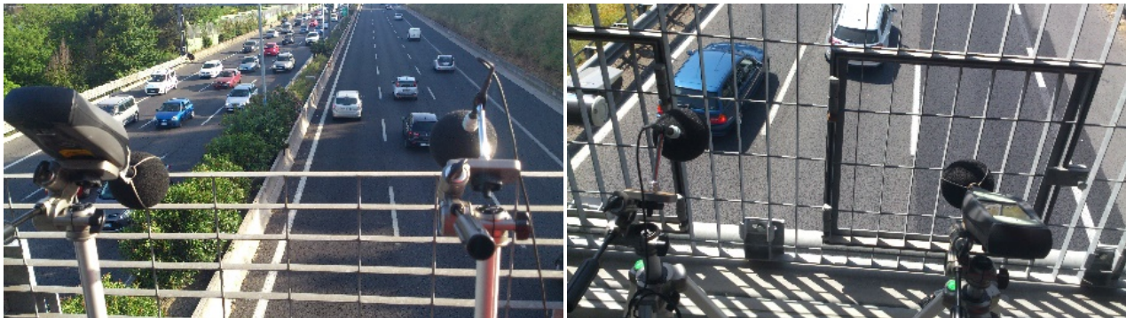
Figure 10: Examples of the recording devices installed in the ANAS S.p.A. portals situated on the A90 highway surrounding Rome [30].
