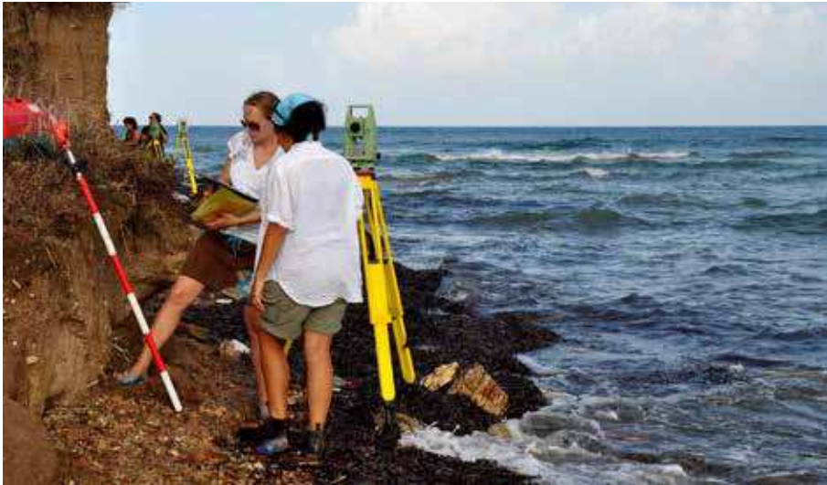
Figure 6.7: Kyllene Harbour Project, 2014-2016. Total station documentation of the cliff face with archaeological layers (image by Jari Pakkanen).
