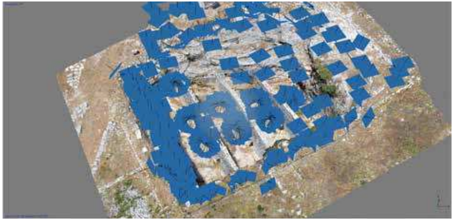
Figure 6.9a: Finnish Institute Three-Dimensional Development Programme, 2016. Hellenistic reservoir at Pleuron. Combining land-based and aerial digital photography to produce three-dimensional models using photogrammetry. Model with locations of the UAV and hand-held camera photographs indicated by blue rectangles (image by Jari Pakkanen).
