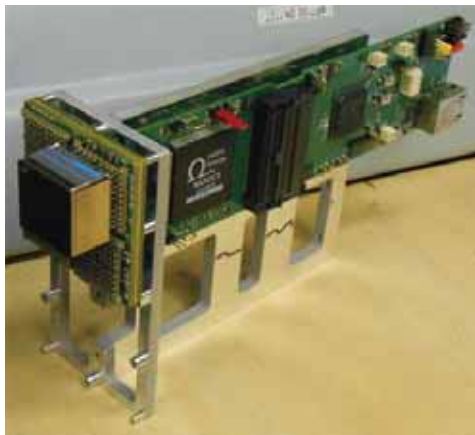
Figure 2.18: A photograph of the LS1 2 \times 2 MaPMT module.
