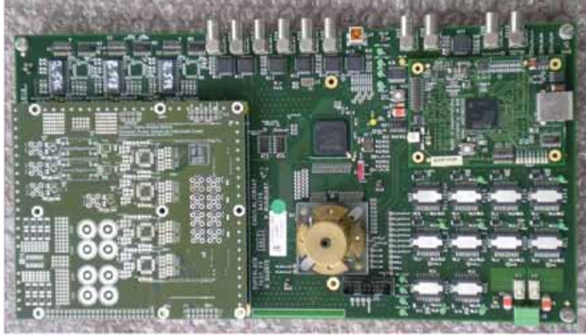
Figure 3.5: Picture of the prototype of the Front-End board. The analogue mezzanine is visible on the left. The two FPGAs (models A3PE and AX from MICROSEMI/ACTEL, see the text) are in the central part of the board, in black and under the copper socket.
