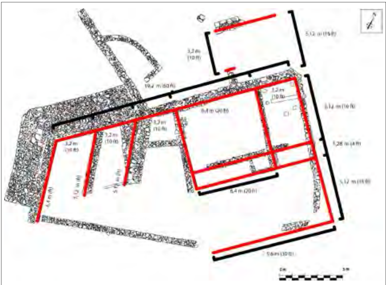
FIGURE 6. Plan of Building A and proposed metrological interpretation based on the use of 0.32 m as the unit of measurement.
