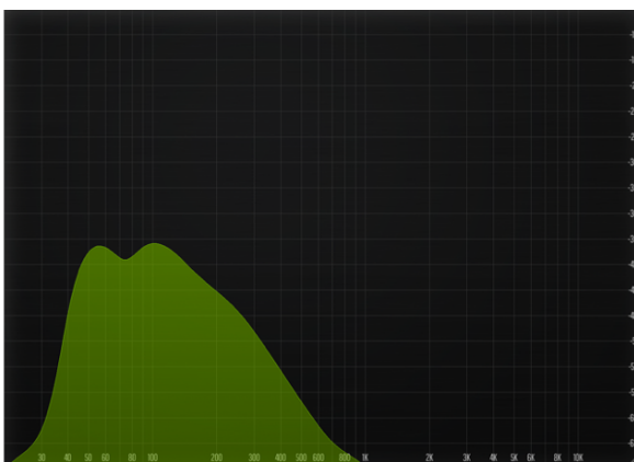
Figure 4.2.2: Bass frequency spectrum on the chorus. We can see a bass dip around 70Hz.
