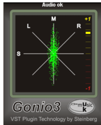
Figure 3.3.5: Lissajous figure. Source: Screenshot of Steinberg's Gonio3 goniometer plugin
